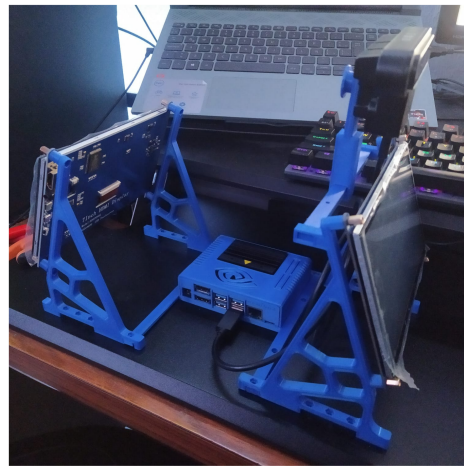
Figure 12. Final Prototype. The image shows the two touchscreens back-to-back with the main processor in the middle.
